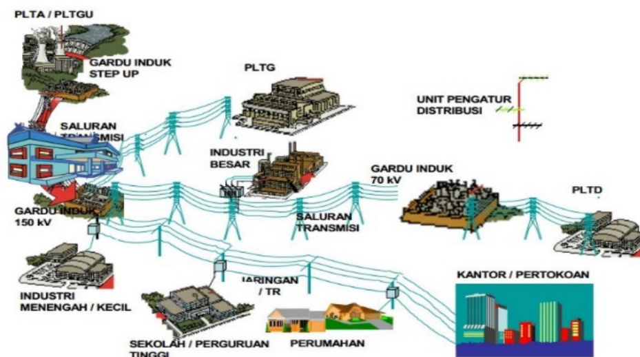
Figure 1. Electric Power Distribution System
