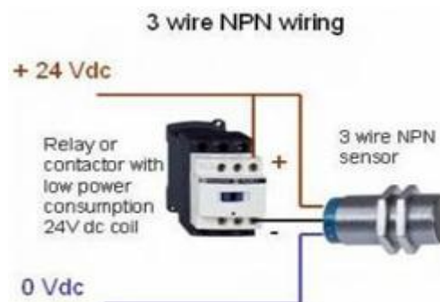
Figure 7. Schematic of the NPN sensor circuit
