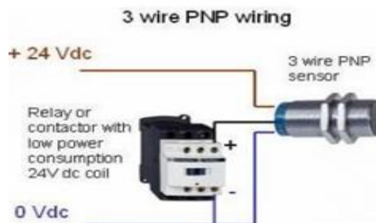
Figure 8. PNP sensor circuit schematic
