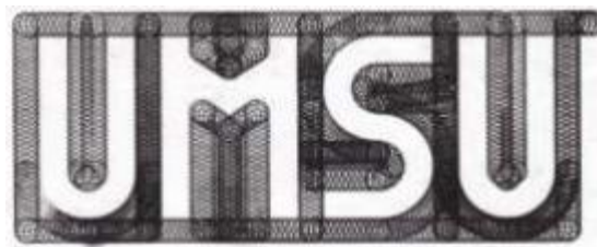
Figure 7. Machining Toolpath of "UMSU" (Rahmatullah, et al, 2021)
